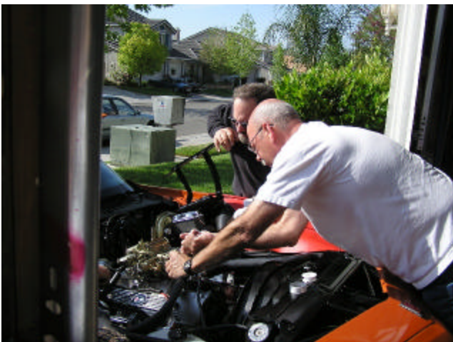
Darrell and Dick adjust the carburetor's idle speed and fuel mixture. The engine almost immediately started up on first try. A make-shift exhaust system with mufflers attached keeps the noise level down.
